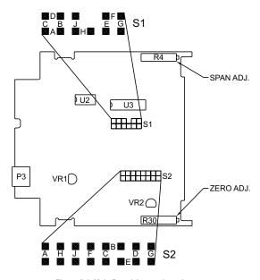
Figure 5-1 Main Board Jumper Locations
